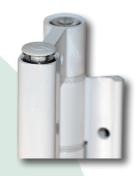
**3)** Using your 6mm Allen key wind the screw anti-clockwise to lift the sash by up to 5mm\*
