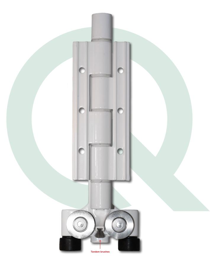
Long life and smooth action are further aided by the integral brushes on all roller assemblies. These clear away any dust or other small debris each time the door is folded open, preventing any major build up that may impede the operation of the door
